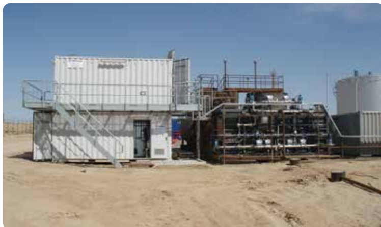
The Flottweg containerised solution including control cabinet, machine container and product feed container.
