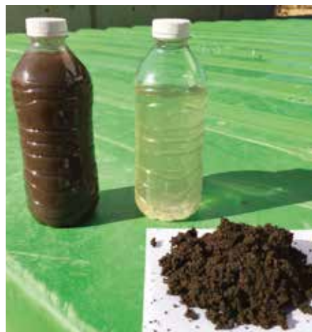
Left: Sludge before dewatering/Right: Centrate after the centrifuge and the discharged solids
